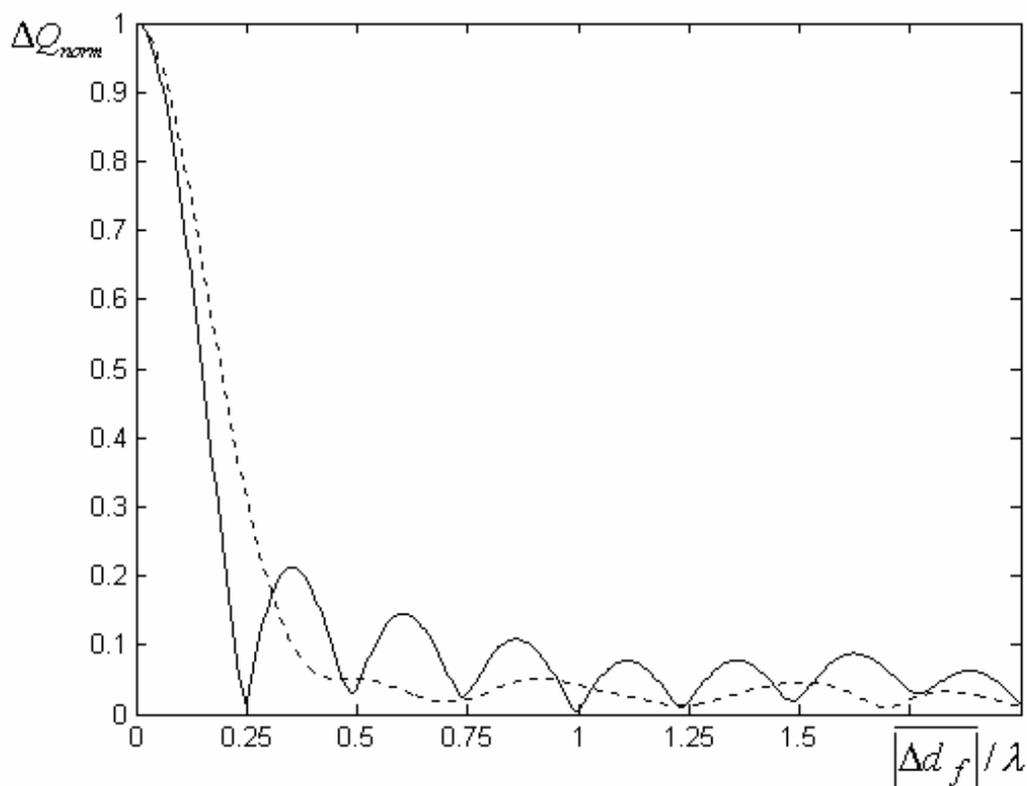
Fig.3. Dependences of an interferential component of response of a photodetector on absolute mean deviation of an optical distance, normalized to a wavelength. The deviation of an optical distance on square of a photodetector is distributed under the uniform law (continuous line) and normal (dashed line) laws.
