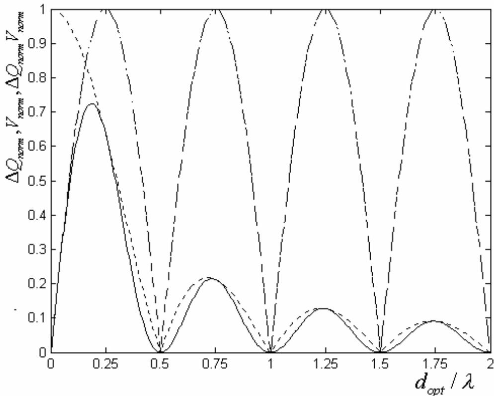
Fig.2. Interference signal of a photodetector  $\Delta Q_{norm}$  (dash-dotted line), contrast  $\zeta_{vopu}$  (dashed line),  $\Delta Q_{norm} V_{norm}$  (continuous line). On an abscissa axis the normalized optical distance of a photoelectric stratum is postponed. The total response of a photodetector is proportional:
