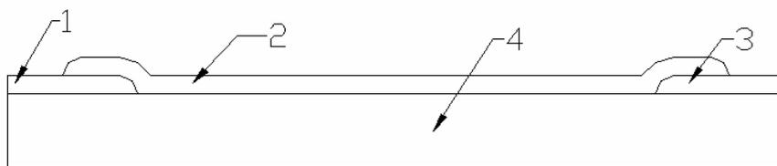
Fig.4. The scheme of an interference responsive photodetector.
