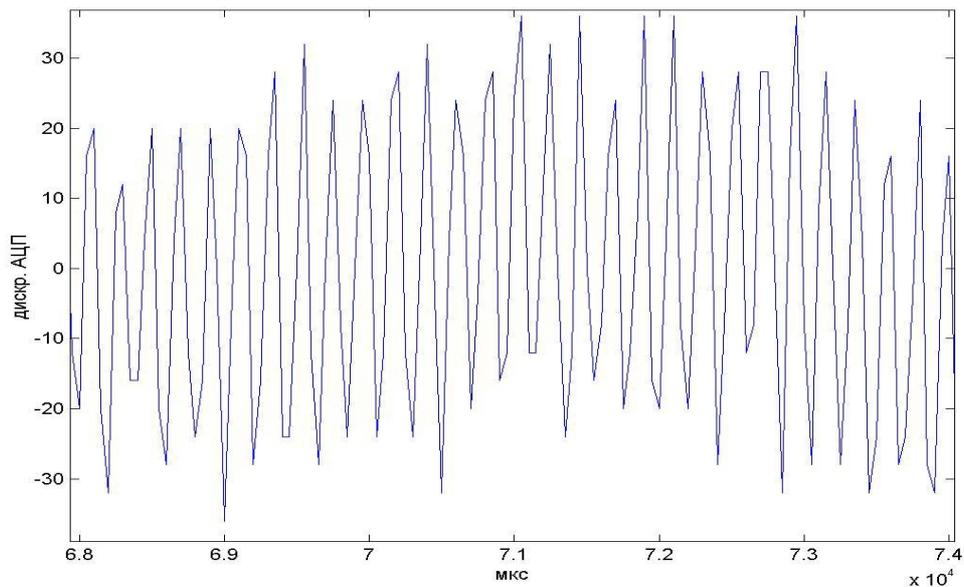
Fig. 5. Response of a photodetector at its uniform driving in an interferential field of counter luminous fluxes He-Ne of the laser.
