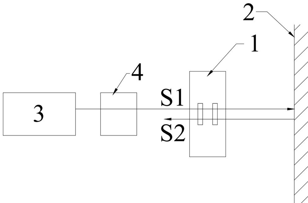
Fig. 7. The scheme of an interferometer . 1 - quadrature photodetector responsive to allocation of an interferential field; 2 - reflector; 3 - He-Ne the laser; 4 - collimator.
